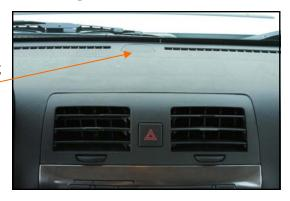
3. With a small screw drive remove dash panel plug.
