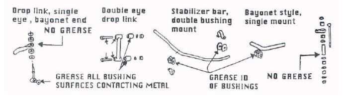
There are many types of stabilizer bars, your vehicle could have any combination of components. Lubricate your new suspension components as shown above. Lubricate track bars as you would double drop links. Use a Teflon based grease on your polyurethane components, it will give you increased performance and longevity.
