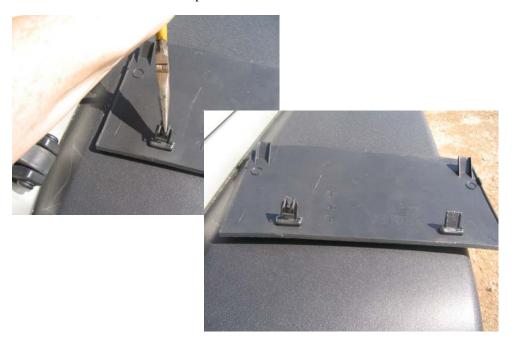
5. With the needle nose pliers compress the clips flat so they will clip on the Daystar switch panel.
