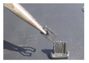
6. Working from the back side of the panel use your razor blade knife and cut out the switch holes. Do not over cut the hole.
