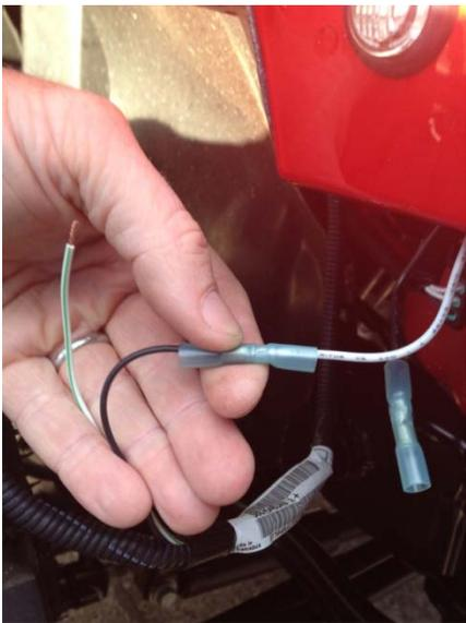
5) Install butt connectors. The LED's are polarity sensitive (will only light with power going one way). This 2014 JK needed wires to be black/white and white/black for the LED's to illuminate. Use a lighter to shrink the butt connectors covers. Tuck wires away, and you are complete.
