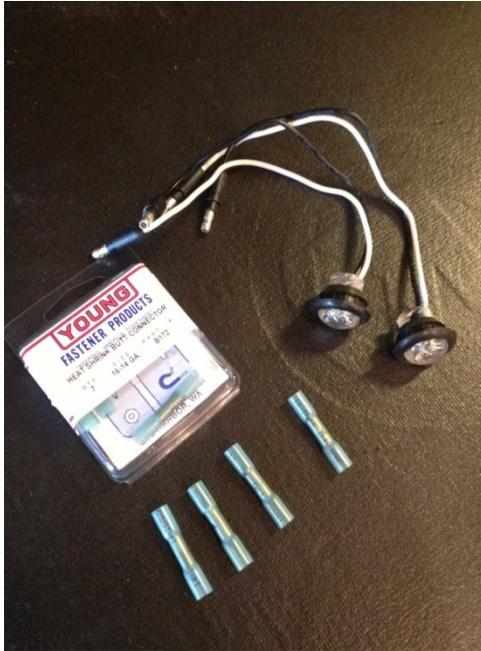
1) Install butt connectors on LED's
