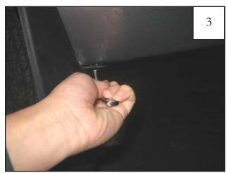
Remove screw from underside of factory mud guard.
