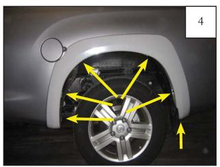
Hold the flare firmly on the fender. Start a supplied Hex Screw through each hole in flare and into hole in fender (six places).
