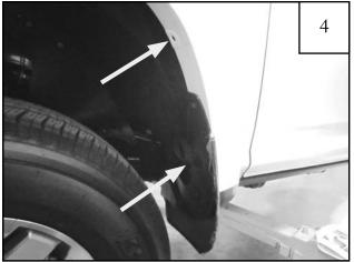
Using a 10mm socket, remove two factory screws located at the rear of the wheel well. Retain screws for reinstallation. **NOTE: Flare are meant to be installed with Factory Mud Flaps. Do not remove mud flap.**
