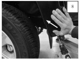
NOTE: When drilling the bottom rear hole of the front flare, push the flare forward and in towards the wheel well.
