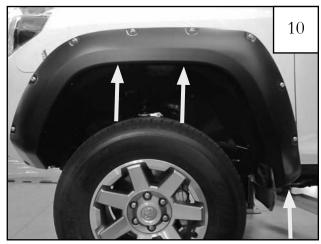
Install supplied push retainer (RV1-P009) into the remaining three holes drilled in the Step 7. Ensure flare is positioned properly, then apply inward pressure on the flare at each hole location while tightening each screw.
