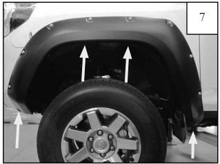
Using a 5/16" bit, drill through holes located at the top center, bottom front and rear of the flare into the plastic where indicated.
