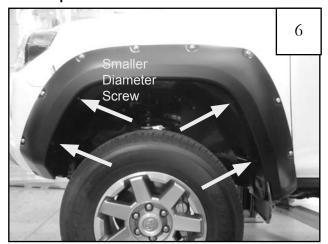
Position Front Flare on Fender temporarily. Reinstall factory screws through flare and into hole locations shown. *NOTE: Make sure the smaller diameter screw is re-installed into the same hole*. Tighten all factory screws.
