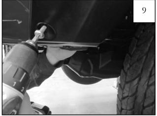
Install supplied bolt (SW1-0041) with one washer (WA1-0012) in bottom front hole of flare. Install nylock nut (NU1-0019) from backside of bumper cover. Tighten with 1/2" wrench.
