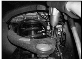
3. Working on the driver side, remove the hardware that connects the brake line bracket to the knuckle. Save the
