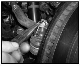
27. Locate the brake line mounting hardware. Working on the driver side, secure the brake line bracket to the knuckle and secure using the OE hardware. Make sure to add some loctite and torque to 12 lbs.
