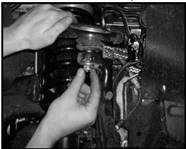
24. Locate the upper control arm cotter pin. Working on the driver side, install the cotter back into the upper control arm ball joint. Special note: If the cotter pin can not be installed because the hole in the castle nut does not line up with the ball joint, DO NOT loosen the castle nut so that the cotter pin can fit, tighten the castle nut some more so that the cotter pin can be installed.
