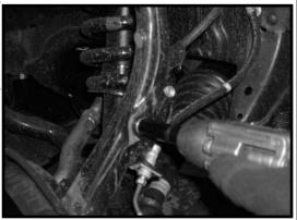
4. Working on the driver side, remove the (4) upper nuts that connect the strut into the upper location. Save the nuts for later re-installation. Repeat procedure on the passenger side. Special note: Only remove the (4) upper outer nuts, DO NOT remove the nut in the middle of the strut.
