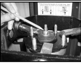
18. Locate (4) S10090 sleeves from hardware bag 52070NB. Locate the (4) upper OE nuts. Also, locate the newly modified strut. Working on the driver side, install the modiffied strut into the upper location and secure using the OE nuts. Do not tighten at this point. Special note: Make sure that the out arrow is facing towards the outside of the vehicle.
