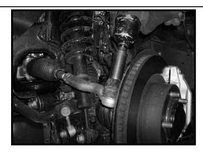
8. Working on the driver side, loosen but do not remove the nut that connects the outer tie rod ball joint to the steering knuckle. Carefully break the taper by striking the knuckle with a hammer. Special note: Take special care not to damage the outer tie rod ball joint dust boot. Repeat procedure on the passenger side.
