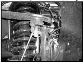
6. Working on the driver side, loosen but do not remove the nut that connects the upper control arm ball joint to the steering knuckle. Carefully break the taper by striking the knuckle with a hammer. Special note: Take special care not to damage the upper control arm ball joint or rip the upper control arm ball joint dust boot. For now, leave the upper control arm attached to the knuckle. We want to just break the taper for now. Repeat procedure on the passenger side.
