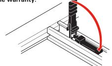
Fold the tonneau forward and fasten the straps in the middle section to the front rail. Check that the straps are tight.
