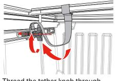
Thread the tether knob through the lock washer, through the tether bracket and into the slide block.
