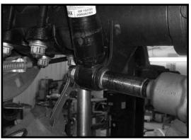
13. Working on the driver side, remove the stock u-bolt from the stock shock into the stock location using the new 12 mm the stock location. The stock u-bolts and hardware may be hardware. Make sure to use thread locker or loctite and discarded. Place the upper and lower u-bolt plates aside. Repeat procedure on the passenger side.
