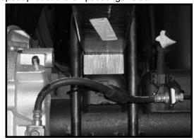
18. Working on the driver side, install the stock shock back into the axle mount using the stock hardware. Make sure to use thread locker or loctite and torque to 75 ft lbs. Repeat procedure on the passenger side.
