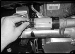
29. Re-install the drive line back to the front differential using the OE hardware. Make sure to use loctite and torque to **35 ft lbs.**
