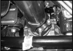
30. Re-install the rear cross member to the driver and passenger side rear lower control arm drop pockets using the OE hardware. Make sure to use loctite and torque to **55 ft lbs**.
