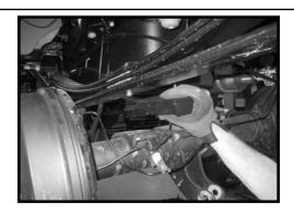
55. Locate (2) new 3" lifted blocks. Working on the driver side, install the new 3" lifted block into the stock location. Repeat procedure on the passenger side.
