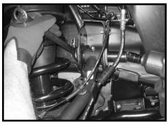
46. Working on the driver side, grease the upper control arm bushings and ball joint. Repeat procedure on the passenger side. Special note to the customer: Make sure to have the upper control arm bushings and ball joints greased each time you have the oil changed.
