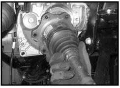
15. Working on the driver side, remove the rear cross memware.
