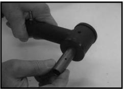
32. Locate (4) SERT04 from hardware bag 14056NB1. have been cut off, remove the OE nuts from each stud. Install the new sert fittings to the new upper control arm. Special note: Take special care not to cross thread during installation and make sure not to over tighten. Hand tighten with an end wrench. Also, make sure that once installed the sert fitting is facing the outside of the vehicle so it will be easy to access with a grease gun.
