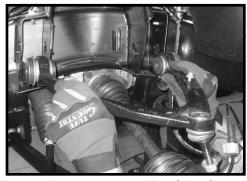
12. Working on the passenger side of the front differential, locate the wiring harness that connects the 4WD control panel to the front differential. Disconnect the 4WD wiring harness from the front differential. Tie the 4WD wiring harness up and out of the way. Special note: Take special ber from the OE location. Save the cross member and hardcare not to kink the wiring.
