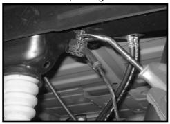
51. Place a pair of hydraulic floor jacks under the rear differential. Carefully raise up on the hydraulic floor jacks until they make contact with the rear differential.
