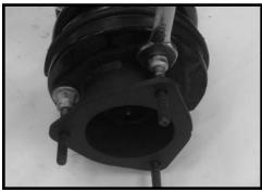
36. Locate (6) 3/8" nylon lock nuts and (6) 5/16" USS flat washers from hardware bag 14056NB2. Working on the driver side, install the newly modified strut into the upper location and secure using the new hardware. Make sure to use loctite and torque to 35 ft lbs. Repeat procedure on the passenger side.
