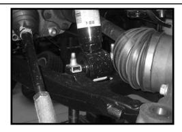
8. Working on the driver side, remove the upper clips off the upper strut studs. Remove the nuts holding the strut into the upper location and save. Remove the strut from the vehicle and remove and discard the lower attaching clips. Set the strut aside. Repeat procedure on the passenger side.
