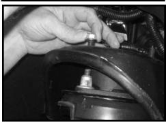
37. Locate (4) 10 mm x 55 mm bolts and (4) 10 mm unitorque nuts from hardware bag 14056NB1. Locate (8) 10 mm flat washers from hardware bag 14056NB2. Working on the driver side, secure the lower portion of the OE strut to the lower control arm using the new hardware. Make sure to use loctite and torque to 45 ft lbs. Repeat procedure on the passenger side.
