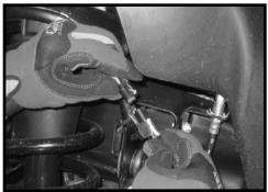
4. Working on the driver side, remove the ABS line from the OE upper control arm. The hardware maybe discarded. Carefully remove the bracket from the ABS line and brake line and set aside. Repeat procedure on the passenger side.
