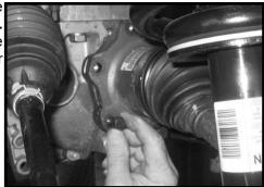
nuts from hardware bag 14056NB2. Working on the driver sure to use loctite and torque to 40 ft lbs. side, re-connect the ABS lines back together. Install the ABS line and brake line back into the OE bracket then secure the OE bracket to the new 6 mm bolt on the upper control arm using the new hardware. Make sure to use loctite and hand tighten with a wrench. Also, install the ABS line back to the frame rail. Repeat procedure on the passenger side.
