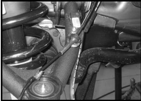
41. Working on the driver side, install the outer tie rod to the OE knuckle using the OE hardware. Make sure to use loctite and torque to **95 ft lbs.** Repeat procedure on the passenger side.
