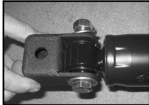
59. Working on the driver side, install the modified shock into the upper and lower location using the OE hardware. Make sure to use loctite and torque to **85 ft lbs**. Move back to the new 9/16" hardware and add some loctite and torque to **85 ft lbs**. Repeat procedure on the passenger side.
