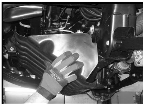
3. Working on the driver side, remove the ABS line from the bracket on the top of the upper control arm pocket. Now disconnect the ABS lines from each other at the quick disconnect. **Special note: Take special care not to damage ABS line during removal.** Repeat procedure on the passenger side.
