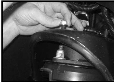
37. Locate (4) 10 mm x 55 mm bolts and (4) 10 mm uni-torque nuts from hardware bag 14056NB1. Locate (8) 10 mm flat washers from hardware bag 14056NB2. Working on the driver side, secure the lower portion of the OE strut to the lower control arm using the new hardware. Make sure to use loctite and torque to **45 ft lbs**. Repeat procedure on the passenger side.
