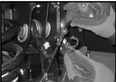
5. Working on the driver side, remove the sway bar end link from the sway bar and lower control arm. Save the end link and hardware. Repeat procedure on the passenger side.
