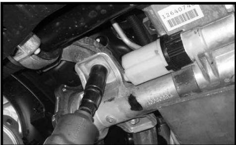
18. With the help from a buddy, carefully remove the front differential from the vehicle and set it on the ground or a work bench.
