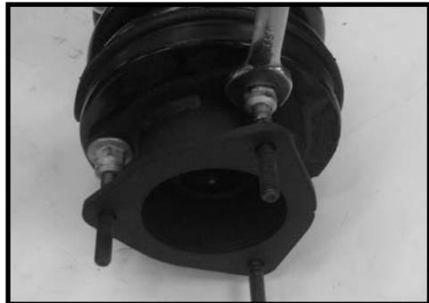
36. Locate (6) 3/8" nylon lock nuts and (6) 5/16" USS flat washers from hardware bag 14056NB2. Working on the driver side, install the newly modified strut into the upper location and secure using the new hardware. Make sure to use loctite and torque to **35 ft lbs**. Repeat procedure on the passenger side.
