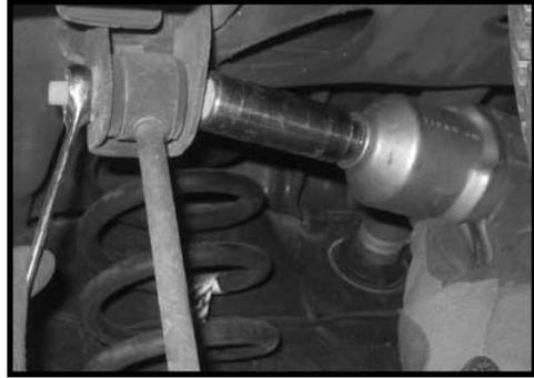
54. Working on the driver side, remove the track bar from the OE track bar mount. Save the hardware for later re-installation.
