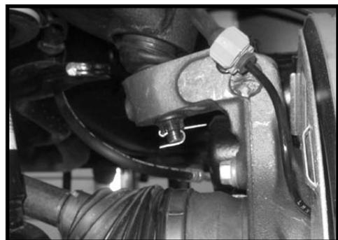
39. Working on the driver side, re-install the CV axle to the front differential using the OE hardware. Make sure to use loctite and torque to **45 ft lbs**. Repeat procedure on the passenger side.
