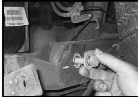
55. Carefully lower down both hydraulic floor jacks at the same time approximately 3". **Special note: Take special care not to over extend any brake lines and/or hoses.** Working on the driver side, remove the coil spring and set aside. Repeat procedure on the passenger side.
