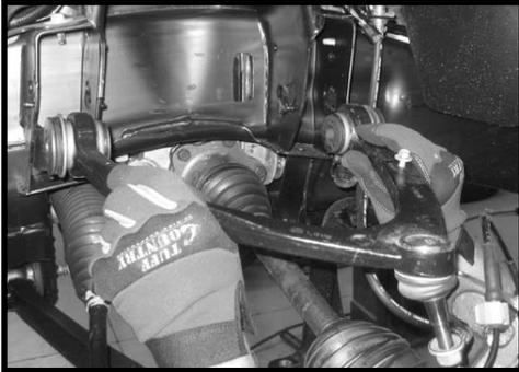
12. Working on the passenger side of the front differential, locate the wiring harness that connects the 4WD control panel to the front differential. Disconnect the 4WD wiring harness from the front differential. Tie the 4WD wiring harness up and out of the way. **Special note: Take special care not to kink the wiring.**
