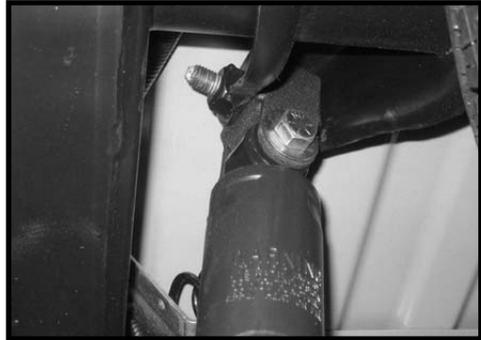
60. Locate the new zip tie in hardware bag 14058NB1. Working on the driver side, zip tie the ABS line to the OE bump stop bracket. Repeat procedure on the passenger side.
