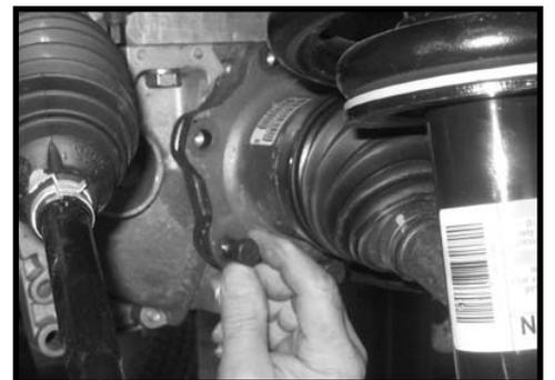
40. Locate (2) 6 mm flat washers and (2) 6 mm unitorque nuts from hardware bag 14056NB2. Working on the driver side, re-connect the ABS lines back together. Install the ABS line and brake line back into the OE bracket then secure the OE bracket to the new 6 mm bolt on the upper control arm using the new hardware. Make sure to use loctite and hand tighten with a wrench. Also, install the ABS line back to the frame rail. Repeat procedure on the passenger side.
