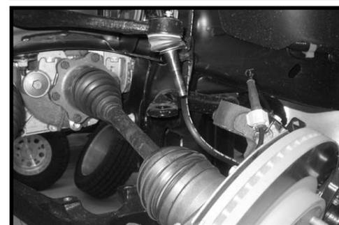
11. Working on the driver side, remove the upper control arm from the upper control arm location. The upper control arm may be discarded but save the upper control arm hardware. Repeat procedure on the passenger side.
