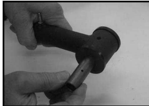
32. Locate (4) SERT04 from hardware bag 14056NB1. Install the new sert fittings to the new upper control arm. **Special note: Take special care not to cross thread during installation and make sure not to over tighten. Hand tighten with an end wrench. Also, make sure that once installed the sert fitting is facing the outside of the vehicle so it will be easy to access with a grease gun.**
