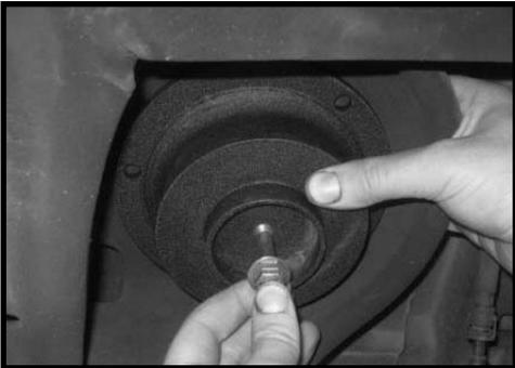
57. Working on the driver side, locate and install the coil spring back into the vehicle. Install the upper portion to the newly installed coil spring and lower lower portion to the axle. Carefully raise up on the hydraulic floor jack until the coil springs seats properly into the vehicle. Repeat procedure on the passenger side.
