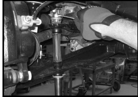
6. Working on the driver side, remove the outer tie rod from the OE knuckle. Save the hardware. **Special note: Using a hammer and striking the knuckle will help break the taper. Take special care not to damage the outer tie rod dust boot during removal.** Repeat procedure on the passenger side.
