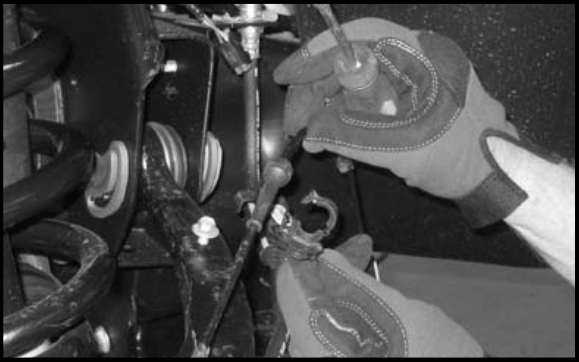
14. Working on the driver side, remove the sway bar end link from the sway bar and lower control arm. Save the end link and hardware. Repeat procedure on the passenger side.
