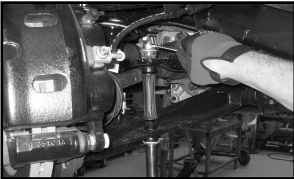
14. Working on the driver side, remove the sway bar end link from the sway bar and lower control arm. Save the end link and hardware. Repeat procedure on the passenger side.
