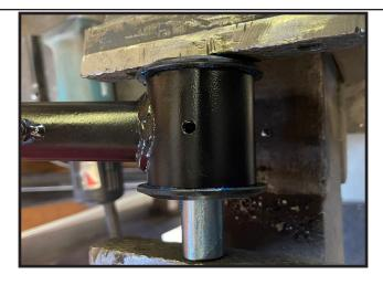
14. Carefully install the grease fittings into the threaded holes of the upper control arms. **Be careful to not over tighten these as they are made of brass and can easily strip out.**
