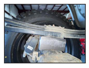
6. Secure using the new u-bolts and hardware. **Snug the up-bolts at this time but do not fully torque yet.**
