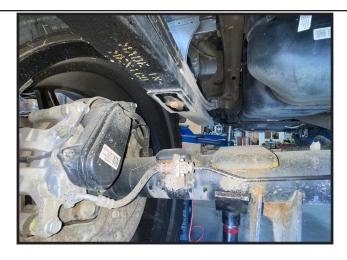
5. Install the new lift block between the bottom of the leaf spring and the perch on the axle making sure alignment pin and hole are lined up.
