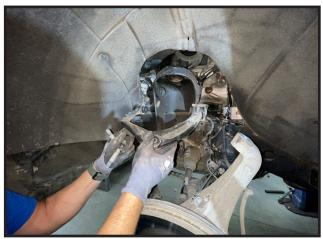
13. Locate the new Driver side upper control arm, also locate (4) Polyurethane bushings, (2) crush sleeves, and (2) grease fittings. Using a polyurethane compatible grease, apply a healthy amount on the bushings and crush sleeves, then install into the new upper control arms.
