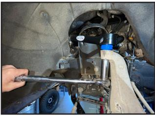
mark the orientation of the components so that it can be lower coil spring perch and discard. re-assembled in the same place.
