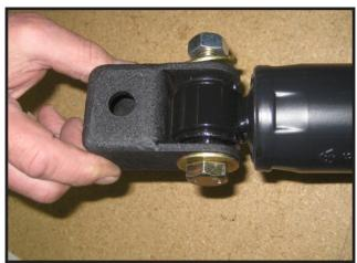
10. Re-install shocks using the OE hardware.
