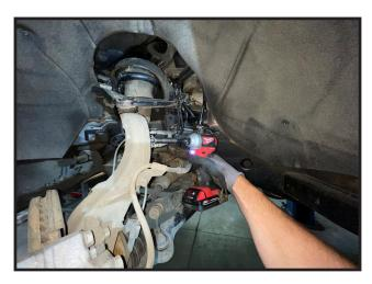
4. Remove the lower control arm mounting bolts and hardware and save.
