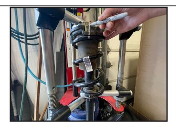
20. Relieve the pressure from the strut top hat, remove the OE nut, top hat, and coil spring. Save hardware for later
