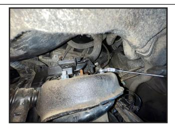
7. Once upper hardware is removed, carefully remove the strut from the vehicle and set aside
