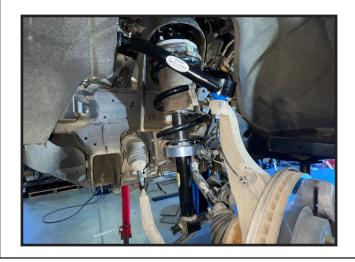
31. Locate (2) 10mm x 60mm bolts, (4) 10mm flat washers, and (2) 10mm unitorque nuts. Carefully raise up the lower control arm so that the lower strut mounting points are lined up and install the new 10mm hardware with the bolt heads facing up. **Do not tighten at this time.**
