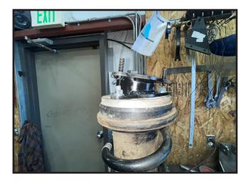
29. While the strut is still on the bench, Remove the (2) OE clip nuts from the bottom mount of the shock and discard.
