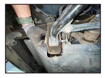
5. Working on the lower strut mount, remove the 2 bolts that attach it to the lower control arm. Special note: when these bolts are out, be careful that the lower control arm doesn't drop and swing away too fast and damage anything.
