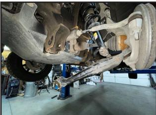
6. Now move to the upper strut mount and remove the 3 nuts that attach the strut to the mount while holding onto the strut so it doesn't drop out.
