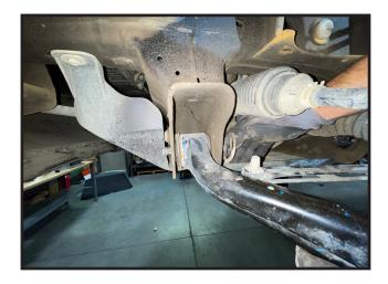
9. Remove the ABS wire harness mounting bracket from the upper control arm and pull aside.
