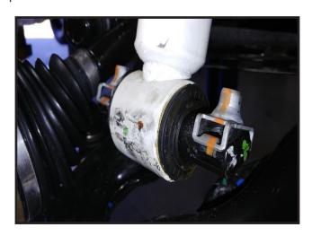
30. Locate (3) 3/8" flange nuts, Install the strut assembly back on the outer most upper stud.
