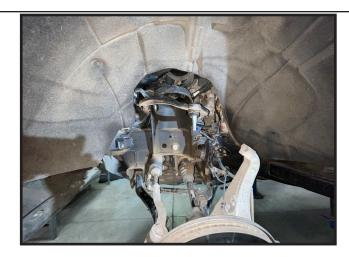
12. Remove the 2 bolts and hardware that attach the upper control arm to the vehicle, and remove the OE upper control arm.
