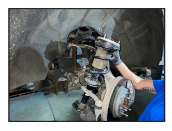
8. Move back to the lower control arm and re-install it into its mounting pockets using the OE bolts. No need to tighten the bolts, they are just to hold it in place for now.
