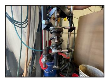
26. Take the strut assembly out of the compressing tool and take it to the bench. Install the new supplied 10mm flange nuts and thread them all the way down on the 3 studs on top of the strut. Using a cutting tool, cut 1/4" (roughly 3-4 threads) off of the top of the 2 outer OE studs to make them short enough to clear the new strut spacer. Next cut the 1 into the vehicle and loosely start only 1 of the 3/8" flange nuts inner stud off flush with the top of the flange nut
