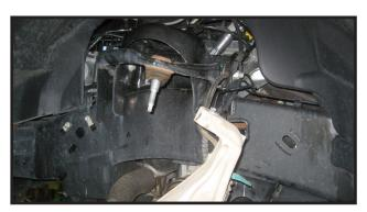
11. Remove the upper control arm from the vehicle, saving the hardware for later re-installation.
