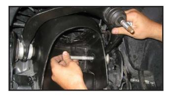
12. Locate the new driver side upper control arm part # 23925-01. Also locate (4) TC-002 bushings, (2) S10236 crush sleeves, and (2) SERT06 grease fittings. Install the bushings and sleeves into the new upper control arm. Special note: Make sure to use a fair amount of lithium or moly base grease before installing the new bushings and sleeves, this will increase the life of the bushing as well as help prevent squeaking.
