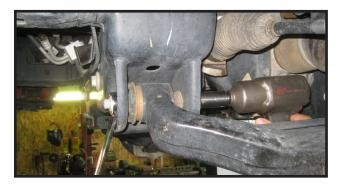
21. Return to the nuts on the upper strut mount and tighten them down. torque to 45 ft lbs.
