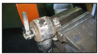
18. With the studs removed from the lower strut mount, you will now be able to re-install the strut assembly back into the vehicle. Locate the OE upper strut mount nuts. Loosely start the nuts on the upper strut mount so the strut can still be maneuvered around. Note: It is usually neccessary to un-pin the lower control arm from the frame pockets again, to allow enough room to install the strut.
