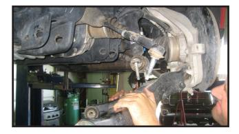
Remove the (3) mounting nuts on the upper strut mount and remove the strut from the vehicle. Set strut assembly aside.
