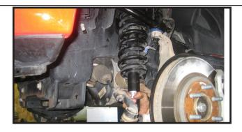
19. Line the lower strut mount up with its mounting holes on 22. Re-install the tie rod end into the steering knuckle and the lower control arm and re-install the (2) studs. Use the torque nut to 95 ft lbs. nuts to tighten and suck the studs back down into the mount.
