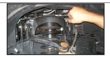
23. Wait to re-install the Sway bar endlink until this process has be performed on the passenger side, then re-install both sway bar endlinks.
