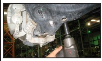
6. Remove the 2 bolts that connect the lower control arm to its pocket mounts on the frame rail.
