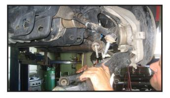
Remove the (3) mounting nuts on the upper strut mount and remove the strut from the vehicle. Set strut assembly aside.
