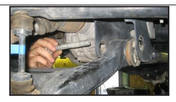
7. At this point, the lower control arm will need to be dropped down away from the lower strut mount. Be extra careful to not over extend any brakelines or the CV axle while performing this step.
