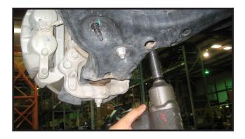
6. Remove the 2 bolts that connect the lower control arm to its pocket mounts on the frame rail.
