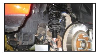
19. Line the lower strut mount up with its mounting holes on the lower control arm and re-install the (2) studs. Use the nuts to tighten and suck the studs back down into the mount.
