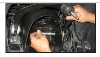
12. Locate the new driver side upper control arm part # 20930-11. Also locate (4) TC-002 bushings, (2) S10236 crush sleeves, and (2) SERT06 grease fittings. Install the bushings and sleeves into the new upper control arm. Special note: Make sure to use a fair amount of lithium or moly base grease before installing the new bushings and sleeves, this will increase the life of the bushing as well as help prevent squeaking.
