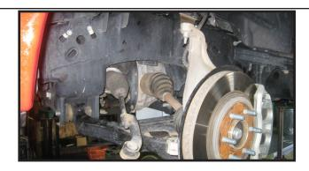
10. Remove the nut from the upper ball joint where it attaches to the steering knuckle. Carefully seperate the ball joint from the steering knuckle by striking the knuckle with a hammer.
