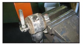
18. With the studs removed from the lower strut mount, you will now be able to re-install the strut assembly back into the vehicle. Locate the OE upper strut mounting hardware and Loosely start the nuts on the upper strut mount so the strut can still be maneuvered around. Note: It is usually neccessary to un-pin the lower control arm from the frame pockets again, to allow enough room to install the strut.
