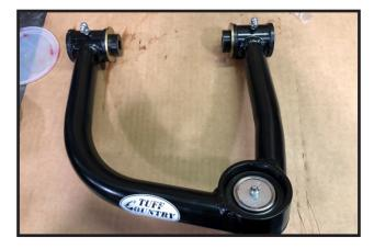
33. Install the grease fittings into each eyelet of the upper control arm. Take special care to not over tighten the fittings.
