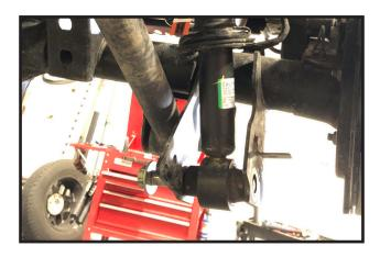
56. Working on the passenger side where the track bar is mounted to the axle bracket, remove the OE bolt and set aside.
