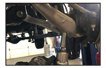
42. Finish installing the 3/8" flange nuts on the top of the strut and torque to 35 ft lbs.
