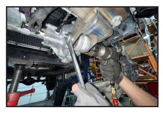
13. Re-install the OE hardware for the heat exchanger that was removed in Step #4
