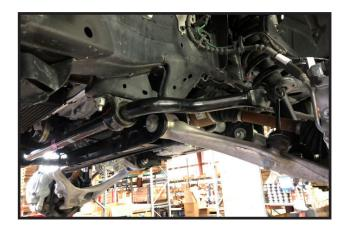
41. Move back to the lower strut mount and tighten the nuts. 44. Make sure to grease the grease fittings at the upper control arm eyelets, and upper ball joints.
