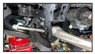
lower strut mounts. Remove the remaining nut on the top top hat. Remove the top hat only and rotate 180 degrees, strut mount and remove struts.
