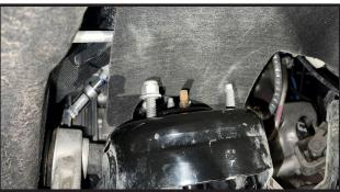
15. Remove the lower sway bar endlink hardware on the driver and passenger lower control arms. Remove the hardware securing the sway bar to the frame and remove the sway bar.
