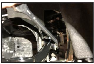
35. Using the new castle nut, washer and cotter pin, secure the upper ball joint to the steering knuckle.
