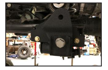
60. Using the new bracket as a guide, drill (2) 3/8" holes into 62. Line the track bar up with the newly installed bracket and install (1) 5/8" x 4" bolt, (2) 9/16" flat washers, and (1) 5/8" unitorque nut.
