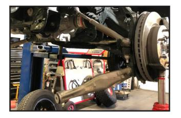
38. Locate 3 new 3/8" flange nuts, install the strut assembly back into the vehicle and LOOSELY start only 1 of the flange nuts.
