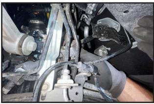
29. Pop out the plastic body clips holding the inner splash guard to the frame rail to gain access to the front upper control arm bolt.
