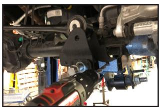
61. In each of the newly drilled holes, install (1) 3/8" x 1" bolt, (1) 5/16" flat washer, and (1) 3/8" flange nut.
