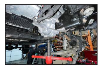
6. Remove the bolt holding the front differential to cross-
