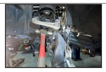
26. Fully remove the upper ball joint nut and seperate the ball joint from the steering knuckle.
