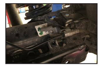
58. Locate the new rear brake line relocation bracket along with (1) 5/16" x 1" bolt, (1) 1/4" flat washer, and (1) 5/16" flange nut. Install the bracket using the OE bolt on the axle mount and the new bolt with hardware on the brake line bracket.
