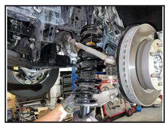
19. Remove the guide pin from the strut top hat.
