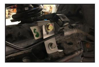
59. Locate the new rear track bar bracket part #23500-06 and place it to the inside of the OE axle bracket. Use the OE bolt to hold in place for now.
