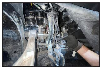
31. Remove the upper control arm from the vehicle.
