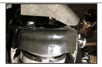
39. Swing the lower control arm back up so that you can start the 2 lower nuts on the strut.
