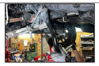
16. Remove the lower strut mounting hardware on the driver and passenger side.
