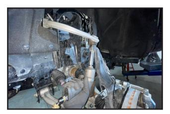
25. Using a hammer, carefully strike the top part of the steering knuckle where the ball joint is installed, You will need to hit this part until the ball joint pops loose.
