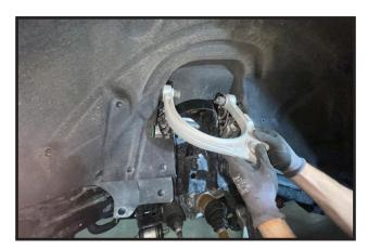
32. Locate the new driver side upper control arm Part #23500-01. Using the diagram below, install the bushings, washers and sleeves. **Make sure to apply grease to the bushings before installing them.**
