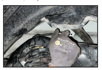
51. Remove the lower mounting bolts and carefully remove the struts from the vehicle.
