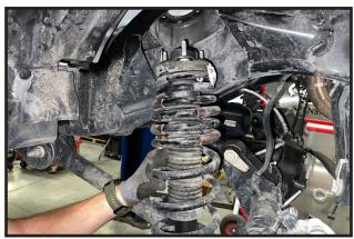
52. Using pliers, remove the dowel pin from the top of the strut hats.
