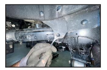
30. Remove the OE upper control arm bolt and set aside.
