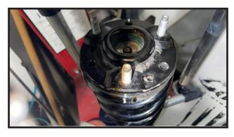
21. Locate part # 22500-01, Install on top of the front sruts using OE hardware. Torque nuts to 85 ft lbs
