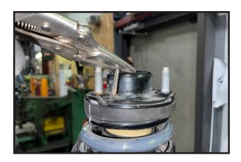
53. Locate and install the new rear strut spacers on top of the OE struts using the OE hardware.
