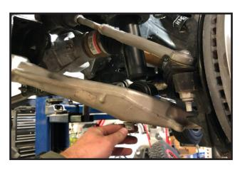
40. Re-install the lower control arm mounting bolts, washers, and nuts. **Do Not tighten at this time.**
