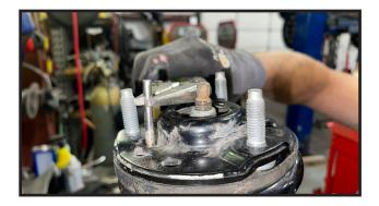
18. Remove lower control arms from mounting pockets and 20. Using a strut spring compressor, Remove the nut on the so there is now lined up to the mark on the coil spring and isolater. Re compress spring and re-install nut, Torque to 80 ft lbs.
