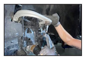
Remove the small phillips head screw from the inner fender liner to access the steering shaft.
