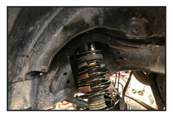
55. Working on the lower mount for the strut, start the OE bolt but do not tighten yet.
