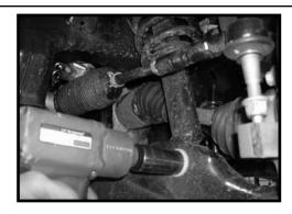
8. Working on the driver side, loosen but do not remove the passenger side. (2) bolts holding the lower control arm to the vehicle. Repeat on passenger side. **Special note: This is done so that the** 13. Re-connect the upper ball joint into the steering knuckle use of a pry bar may make removal easier.
