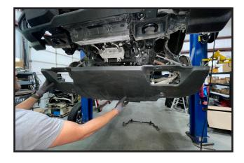
3. Next, remove the steel skid plate from the bottom of the member mount. front and rear cross members. Set aside.
