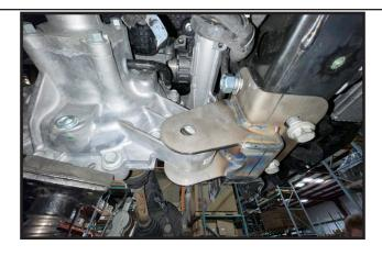
10. Carefully lower the front differential down slightly, and locate the new spacer sleeve, 10mm x 90mm bolt, and over sized washer, Install the spacer sleeve on the passenger side differential mount so that it is spacing the entire front differential down. Start but do not tighten the new 10mm x 90mm bolt with the over sized washer. **Note: photo below shows OE bolt and washer, do not use the OE bolt and washer.**
