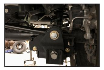
66. Torque the OE bolt to manufacturer's spec's. Torque the new 3/8" bolts to **35 ft lbs**, and torque the new 5/8" bolt to 125 ft lbs.
