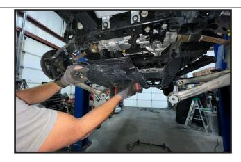
remove the 4 mounting bolts. ( 2 on top, and 2 on bottom ).
