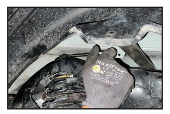
54. Remove the lower mounting bolts and carefully remove the struts from the vehicle.
