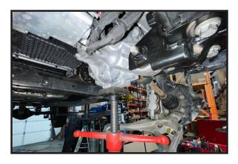
6. Remove the bolt holding the front differential to cross-
