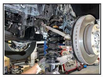
19. Remove the guide pin from the strut top hat. Looking at where the coil spring ends, mark a line on the spring, Isolator 21. Install the new strut preload spacer on top of the OE and top hat, on the center of the 2 studs.
