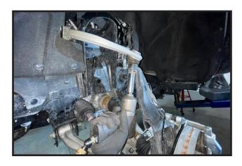
ing knuckle where the ball joint is installed, You will need to turn the steering wheel while this piece is disconnected, hit this part until the ball joint pops loose.
