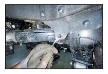
34. Remove the OE upper control arm bolt and set aside.
