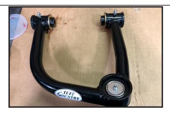
37. Install the grease fittings into each eyelet of the upper 39. Using the new castle nut, washer and cotter pin, secure control arm. Take special care to not over tighten the the upper ball joint to the steering knuckle. fittings.
