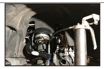
49. Re-install the plastic and steel front skidplates using the OE hardware. Note: the mounting location on the front differential bracket will no longer be used.
