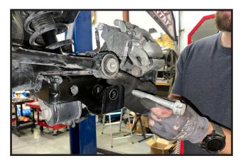
60. Remove the bolt that is holding the rubber brake line 63. Using the new bracket as a guide, drill (2) 3/8" holes into bracket to the track bar bracket and carefully lift the brake the OE axle bracket. hard line up about 2 inches.
