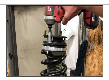
25. Locate the new 1/4" thick top spacer plate and place it over the top of the new strut spacer.
