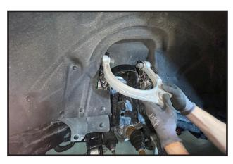
36. Locate the new driver side upper control arm Part #23500-01. Using the diagram below, install the bushings, washers and sleeves. Make sure to apply grease to the bushings before installing them.
