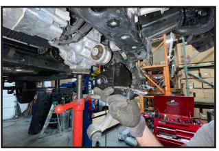
8. Locate and remove the passenger side differential mounting bolt. Special Note: Once this bolt is removed, the front differential will be able to move freely, be careful to not let it fall off of the jack.
