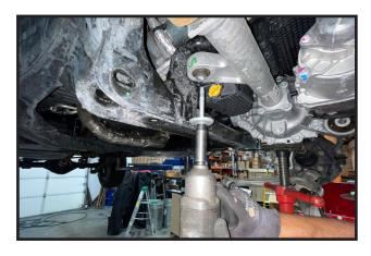
9. Install the new driver side differential bracket. Use the OE bolts that go into the bottom of the crossmember, and use the OE bolt with NEW nut and washer for the through bolt. Leave hardware loose at this time.
