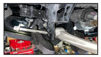
18. Remove lower control arms from mounting pockets and lower strut mounts. Remove the remaining nut on the top
