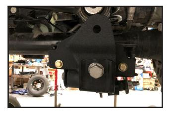
65. Line the track bar up with the newly installed bracket and install (1) 5/8" x 4" bolt, (2) 9/16" flat washers, and (1) 5/8" unitorque nut.
