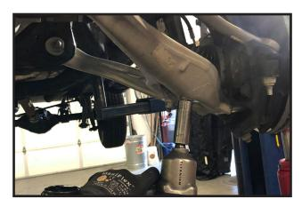
46. Finish installing the 3/8" flange nuts on the top of the strut and torque to **35 ft lbs.**
