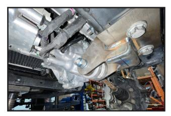
12. Tighten all hardware for the new driver side bracket as well as the 10mm bolt on the passenger side.
