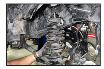
55. Using pliers, remove the dowel pin from the top of the strut hats.
