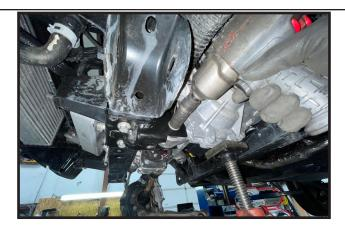
7. Remove the 3 bolts that are holding the differential bracket to the front crossmember and remove the bracket.
