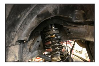
58. Working on the lower mount for the strut, start the OE bolt but do not tighten yet.
