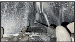
53. Working on the top of the strut, remove the 3 OE nuts. Repeat on the passenger side.
