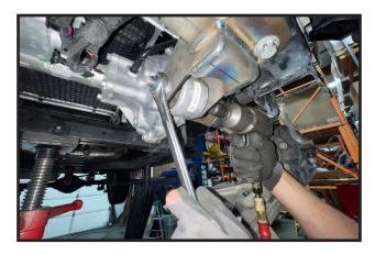
13. Re-install the OE hardware for the heat exchanger that was removed in Step #4
