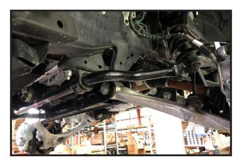
48. Make sure to grease the grease fittings at the upper 50. Install the tires and wheels making sure to torque the lug control arm eyelets, and upper ball joints.
