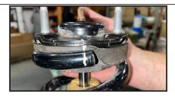
20. Using a strut spring compressor, Remove the nut on the top hat. Lift the top hat off the strut and KEEP the OE rubber isolator in place on top of the coil spring.
