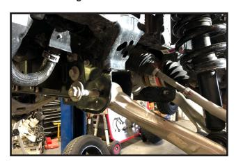
45. Move back to the lower strut mount and tighten the nuts.
