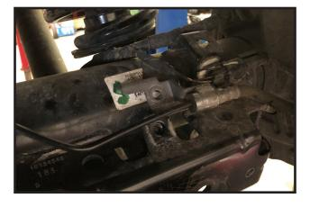
61. Locate the new rear brake line relocation bracket along with (1) 5/16" x 1" bolt, (1) 1/4" flat washer, and (1) 5/16" flange nut. Install the bracket using the OE bolt on the axle mount and the new bolt with hardware on the brake line bracket.
