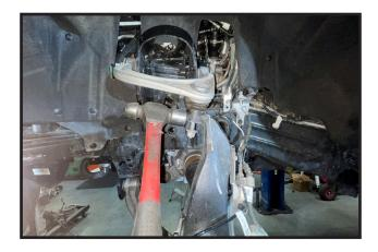
30. Fully remove the upper ball joint nut and seperate the ball joint from the steering knuckle.
