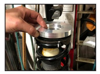
22. Re-install the OE top hat Special Note: Rotate the top hat 180° from the OE position.
