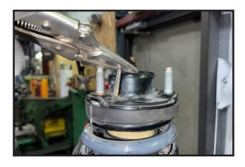
56. Locate and install the new rear strut spacers on top of the OE struts using the OE hardware.
