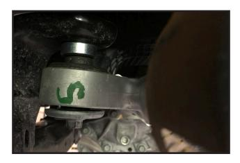
11. Move back to the driver side and start the OE bolt with new nut and washer to mount the differential to the new bracket.
