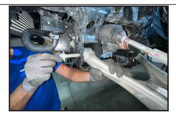
27. Place a floor jack or suitable supporting device under the 31. Remove the small phillips head screw from the inner lower control arm.
