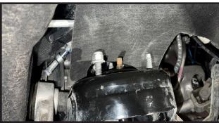
15. Remove the lower sway bar endlink hardware on the driver and passenger lower control arms. Remove the hardware securing the sway bar to the frame and remove the sway bar.
