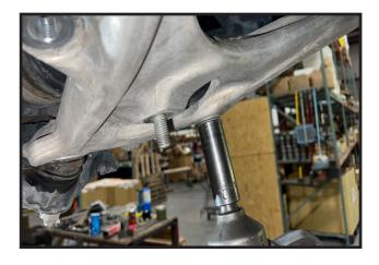
17. Remove lower control arm cam bolt hardware on the driver and passenger side.
