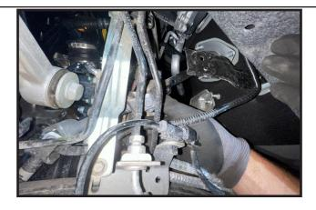
33. Pop out the plastic body clips holding the inner splash 35. Remove the upper control arm from the vehicle. guard to the frame rail to gain access to the front upper control arm bolt.
