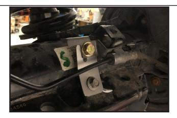
59. Working on the passenger side where the track bar is 62. Locate the new rear track bar bracket part #23500-06 mounted to the axle bracket, remove the OE bolt and set and place it to the inside of the OE axle bracket. Use the OE bolt to hold in place for now.
