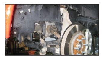
10. Remove the nut from the upper ball joint where it attaches to the steering knuckle. Carefully seperate the ball joint from the steering knuckle by striking the knuckle with a hammer.
