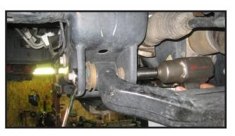
27. Return to the (3) 3/8" nuts on the upper strut mount and tight them down. **torque to 45 ft lbs.**
