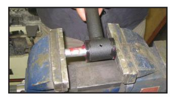
13. Install the new grease fittings into the threaded holes of the eyelets on the upper control arm. Careful to not over Tuff Country Ez-Ride Suspension recommends a wall stripped out.
