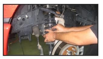
9. Re-attach the lower control arm to the mounting pockets on the frame rail. The bolts only need to be pinned and not tightened, as this is just to hold the lower control arm and steering knuckle up while the new upper control arm is installed.
