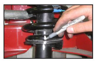
18. Place a clamp on the lower coil spring and mount so tha the shock does not fall to the ground when the nut is removed.
