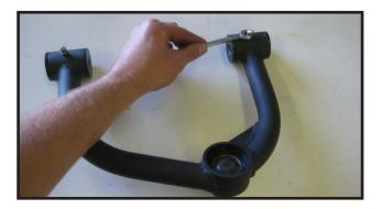
14. Install the new upper control arm into the vehicle using the OE bolts and hardware. Torque to 95 ft lbs.
