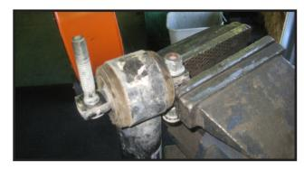
22. Locate a new upper strut spacer part # 22909-01 and install it on the top of the strut using the new M10 serated for a pute. To reue pute to 25 ft the
