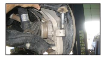
4. Working on the driver side, remove the sway bar endlink
