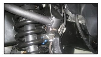
16. At this time it may be necessary to slightly bend the break line mounting bracket that is located on the rear pocket of the upper control arm. This will allow the new upper control arm to fully travel downward.
