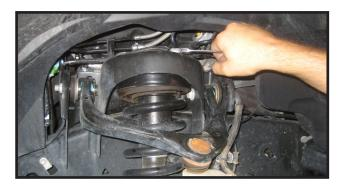
28. Re-install the tie rod end into the steering knuckle and torque nut to 95 ft lbs.
