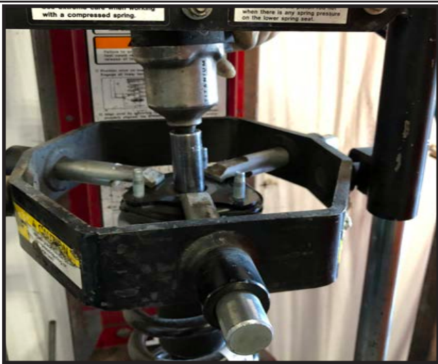
19. Lift off the upper strut plate and set aside.
