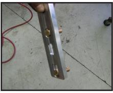
32. With the new 7/16" bolts installed, install the sway bar drop brackets into the OE sway bar locations on the frame using the OE hardware. Torque OE bolts to 40 ft lbs.
