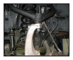
13. Locate (2) 32102-01 bump stop brackets, and (2) 32102-03 bump stop bracket washers from hardware bag 341085NB1. Also locate (2) PB6052 poly bump stops, (2) 5/16" flat washers, and (2) 3/8" nylock nuts from hardware bag 34105NB.
