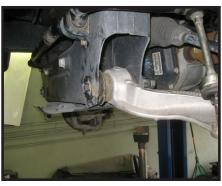
28. Re-install the tie rod ends on each side of the vehicle back into the steering knuckles. Torque to 80 ft lbs.
