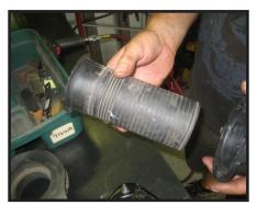
22. Locate the new 34105-04 front strut pre-load spacer and install it into the top strut plate
