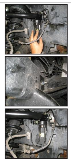
4" bolt through the bracket, through the oblong shaped hole 17. Working on the driver side Lower control arm, remove in the frame, and place the 32102-03 bump stop bracket the 2 bolts connecting it to the frame of the vehicle, carefully washer on the back side. Secure using the 7/16" flat washer and 1/2" unitorque nut. Torque nut to 45 ft lbs and repeat on air. Repeat on passenger side.
