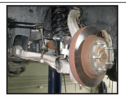
4. Working on the driver side, remove the lower strut mounting bolt and nut, repeat on passenger side.
