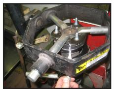
20. Remove the hardware that is attaching the shock to the upper strut plate, then relieve all of the pressure off of the strut so that the top plate can be removed.
