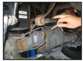
43. Carefully lower the rear axle down enough that the coil springs become loose and can be removed. **Be extra careful to not over extend any brake lines or ABS wire harnesses.**
