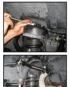
Tuff Country EZ-Ride Suspension recommends a wall mounted strut compressor be used when performing the steps that talk about installing the pre load spacer into the strut. If you do not have a wall mounted strut compressor, please have these steps performed by your local Certified Technician.
