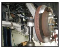
29. Move back to the lower strut mounting hardware and torque to 95 ftlbs.
