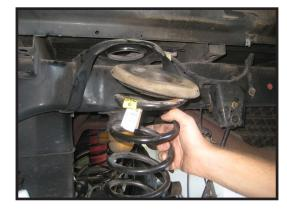
44. Locate (2) 34105-03 rear coil spacers, also locate (2) 7/16" x 1 1/2" bolts, (2) 3/8" flat washers, and (2) 7/16" unitorque nuts from hardware bag 34105NB. Working on the driver side, install the coil spacer into the upper mounting point of the frame and secure it using the new 7/16" hardware. Torque to 42 ft lbs. Repeat on passenger side.
