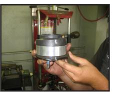
24. Using the wall mounted strut compressor, re-install the strut top plate, preload spacer, and rubber isolator back onto the coil and shock. Secure using the OE hardware and torque to 40 ft lbs.
