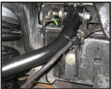
33. Re-install the front swaybar to the newly installed drop brackets and secure using the 7/16" unitorque nuts and 3/8" flat washers. Targue to 40 ft like
