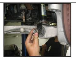
25. Locate the 32902-01 strut spacers and install them on 27. Move back the the lower control arm bolts that were the top of the upper strut plate using the OE hardware. removed in step 17 and re-install. Torque to 105 ft lbs.
