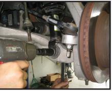
30. Remove the front sway bar from its mounting locations on the frame. Save the OE hardware.
