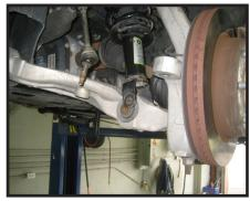
5. Now is a good time to have a jack set up under the lower control arms to support the suspension from dropping suddenly.
