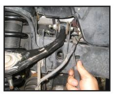
8. Working on the driver side, remove the 2 bolts that are holding the upper control arm on the vehicle, then remove the control arm from the vehicle. Repeat on passenger side.
