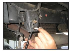
42. Remove the hardware that is attaching the rear Track bar to the axle bracket, save hardware for later installation.
