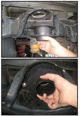
45. Re-install the rear coil springs making sure the OE rubber isolator is between the coil spring and the new coil spring spacer.
