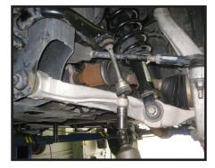
3. Working on the driver side, detach the tie rod end from the steering knuckle by removing the nut, and breaking the taper using a hammer or suitable tie rod removal tool. Repeat on passenger side. **Special note: be extra careful to not damage the tie rod end rubber boot or threads while performing this step.**
