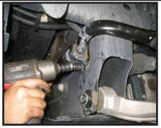
31. Locate (2) 54060-08 sway bar drop brackets, also locate (4) 7/16" x 1 1/2" bolts, (4) 3/8" flat washers, and (4) 7/16"
