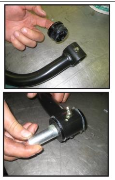
Working on the driver side, Install the new upper control arm into the vehicle using the OE hardware. Torque to 75 ft lbs. Repeat on passenger side.
