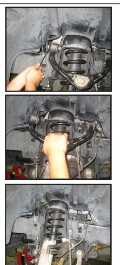
9. Locate the new upper control arms, also locate the (4) grease fittings from hardware bag 34105NB1. Install the grease fittings into each eyelet of the control arms so that they are facing towards the outside of the vehicle. **Special note: Be extra careful not to over tighten these small brass grease fittings**.
