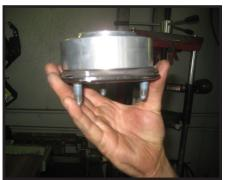
Install the OE rubber isolator onto the newly installed strut pre-load spacer and make sure to line your marks up.
