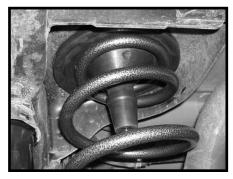
23. Locate (2) 3/8" x 1" bolts, (2) 3/8" lock washers, (2) 3/8" flange nuts from hardware bag 43000NB. Also, locate (2) rear spring retaining washers & (1) 43000-04 nut bracket from hardware bag 43000NB1 Working on the driver side, attach the new rear coil spring retaining washer on the bottom inside of the new coil and secure using the new 3/8" x 1' bolt and hardware and nut bracket. Make sure to use loctite and torque to 18 ft lbs. Repeat procedure on the passenger side.
