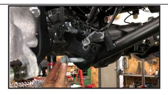
14. Locate (2) of the 516B, (4) 14WA, (2) 516UN. Install the 17. Install the 8MM flang nut and torque to 25 ft lbs. OE brake line bracket on to the brake line mount on the new control arm.
