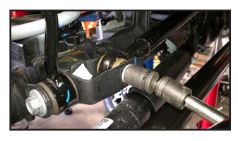
Remove the bolt from the track bar where it attaches to the driver side frame bracket. Save the hardware and remove the entire front track bar.
