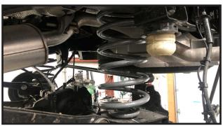
38. Install new rear shocks. Reconect sway bar endlinks and brake line brackets.
