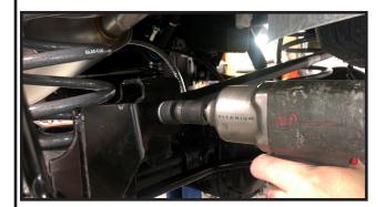
41.Re-install the tires and wheels and torque the lug nuts according to the wheel manufacture's specs. Carefully lower the vehicle back down to the ground.
