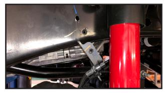
7. Remove both front sway bar end links completely. Save the mounting hardware.
