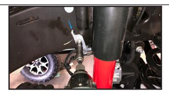
27. Locate (2) of part # S09177-05 Sway bar end link, (4) of part # M02004-BK-01 end link bushings, and (4) of part # S10026 crush sleeves. Install bushing and sleeves into endlinks.
