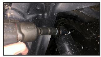
33. Located on the outside of the frame rails, are the brake hose brackets, you will need to remove the bolts that are attaching them to the frame. Save the bolts
