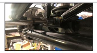
20. With the front track bar installed, tilt it slightly towards the front bumper and tighten the 2 jam nuts on each heim joint
