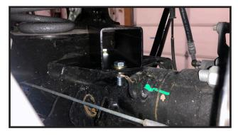
40. Re-install the rear track bar into the pocket using the the OE hardware. **Torque to 125 ft lbs. Special note: You may need to pry the rear axel side to side to line this back up.**
