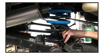
37. Locate (2) of part # GLAD-CL01, Place The OE top spring isolator on top of new coil. Re install new coil springs.
