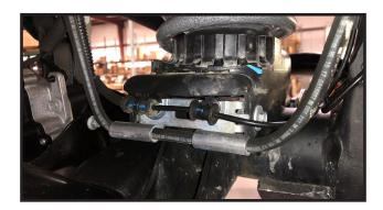
23. Re-install the wire harness plugs/clips to the upper control arms and the frame rails.
