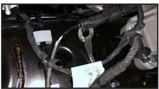
10. Located beneath the front drive shaft, there is a crossmember that is bolted to the bottom of the frame rail on each side, remove the bolts that are holding it to the frame rail and let the crossmember hang from its skid plate.
