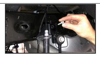
39. Locate (2) of part # 43205-01 rear bump stop extension. (4) 5/16" x 1" bolts, (4) 1/4" flat washers, And (4) 5/16" flang nuts. Install bump stop extension on the rear axle bump stop pad.
