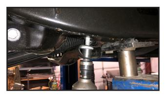
26. Re-install the brake hose brackets to the driver and passenger side frame rails using the OE hardware.
