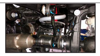
8. Working on the passenger side, locate and remove the brake hose bracket that is attached to the lower coil spring perch. Save hardware
