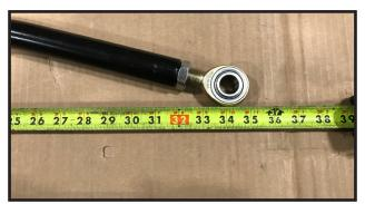
19. Install the S10336 mis-alignment sleeves into each heim joint and install the new track bar in the vehicle using the OE mounting hardware. Torque bolts to 125 ft lbs. Special note, if the track bar does not line up to the mounting holes right away, you may need to pry the axle side to side to get it aligned.
