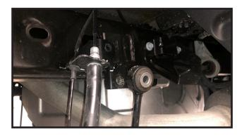
35. Loosen but dont remove upper and lower control arm bolts to help the axle to drop.
