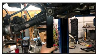
13. Locate the driver lower control arm. Part # S09177-01 and the passenger lower control arm Part # S09177-02. Also locate control arm bushings and sleeves Part # MO9177-BK-01 and Part # S10331. Grease bushings and sleeves and install them into the new control arms. Install Lower control arms. **Torque bolts to 125 ft lbs**.
