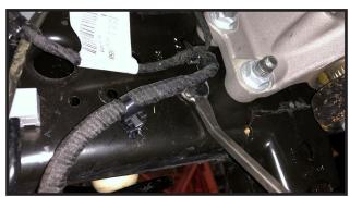
24. Install new front shock absorbers using the OE hardware. Special note: if your new front shocks do not have the proper upper bushings and sleeves already installed in them, make sure to use the new S10325 shock spacer sleeves from hardware bag 43205NB1
