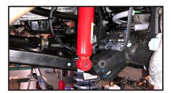
Locate and remove the front brake hose mounting brackets from the driver and passenger side frame rails. Save hardware.
