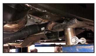
11. With all the slack now obtained in the wire's and brake hoses, carefully lower down the front axle and remove the front coil springs. **Take special care to not over extend any wires or brake hoses.**
