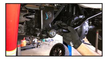
32. Remove both rear shock absorbers, and save the mounting hardware.
