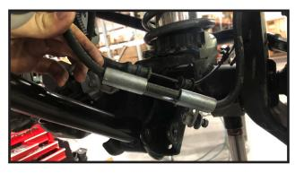
9. To obtain slack in the wire harnesses that control the front axle, you will need to pop out some plastic plugs. these are located on both upper control arms where they mount to the axle, and also up on the inner frame rail if you follow the wires up. Take special care to not damage any wires or plastic plugs as they will get re-installed later on.
