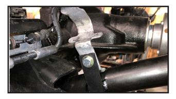
Locate the new front bump stops part # M04001-BK-01. Also locate (2) M8-1.25FLN from hardware bag 43205NB.
