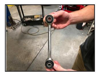
28. Locate (2) 1/2" x 3" bolts, (4) 7/16" flat washers, and (2) 1/2" nuts. Locate the OE lower end link hardware. Install sway bar endlinks. Torque bolts to **65 ft lbs.**
