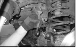
4. Working on the driver side, remove the brake line bracket
