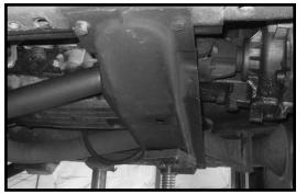
27. Carefully lower down on the on the hydraulic floor jack holding the transfer case cross member about 1 1/2". This will allow enough room for the transfer case spacers to be installed.
