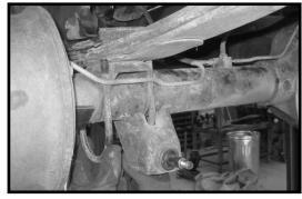
Remove the rear brake line from the OE brake line bracket.
