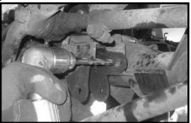
17. Locate (1) 3/8" x 1" bolt, (2) 5/16" USS flat washers and (1) 3/8" unitorque nut from hardware bag 43800NB. Secure the new track bar bracket to the OE bracket using the new 2/9" bardware. Make sure to use loctite and hand tighten with a wrench. Move back to the 5/16" hardware and add some loctite and torque to **18 ft lbs.** Repeat procedure on the passenger side.
