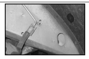
5. Place a pair of hydraulic floor jacks under the front axle and carefully raise up until they make contact with the front axle. Working on the driver side, remove the OE hardware that connects the track bar to the OE location. Save the OE hardware.
