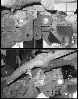
Move back to the OE bolt holding the new track bar **ft lbs.** and wrench tighten the upper hardware. Repeat probracket to the OE pocket and add some loctite and torque to 28 ft lbs.
