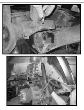
3. Working on the driver side, remove the sway bar endlink from the sway bar and axle location. Save the hardware and endlink. Repeat procedure on the passenger side
