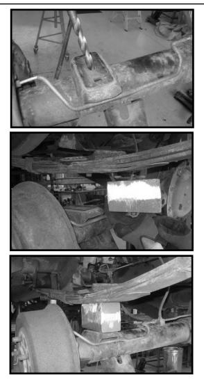
into the OE location using the OE hardware. Make sure to use loctite and torque to lower hardware to **38 ft lbs** and the upper hardware to **12 ft lbs**. Repeat procedure on the passenger side.
