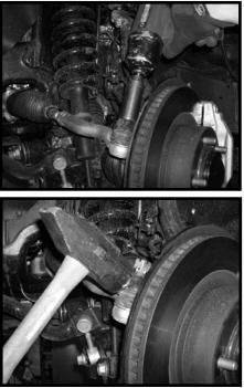
9. Move back to the stock upper control arm ball joint nut and remove completely. Also, move back the stock outer tie rod ball joint nut and remove completely. Remove the stock upper control arm and the stock outer tie rod from the stock knuckle. Let the stock knuckle hang. **Special note: Make sure not to over extend the brake lines, ABS lines and the stock CV axle, if need be, tie the stock knuckle up so these problems do not occur.** Repeat procedure on the passenger side.
