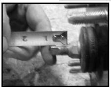
15. Working on the driver side strut, lay the strut on a work bench with the out arrow on the upper strut bearing plate facing the sky. Then scribe a reference mark on the bottom eyelet of the stock strut. This will allow you to install the upper strut plate in the stock location once the strut is put back together with the strut spacer in it.
