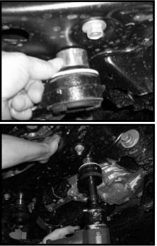
30. Place a pair of hydraulic floor jacks under the front differential. Place one on the driver side and one on the passenger side. Carefully lift up on both hydraulic floor jacks until they make contact with the front differential.
