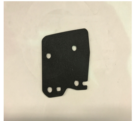
Part # 54050-07 Rear emergency brake cable bracket
