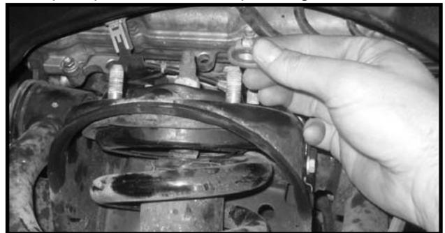
10. Working on the driver side, remove the cotter pin from the castle nut holding the upper control arm to the knuckle. The cotter pin may be discarded. Repeat procedure on the passenger side.
