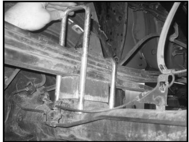
43. Locate the new emergency brake cable extension brackets. Working on the driver side, install the new emergency brake cable bracket to the rear axle using the OE hardware. Do not tighten at this point. Repeat procedure on the passenger side.
