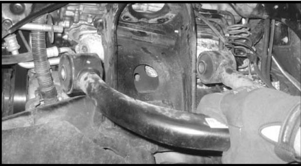
15. Locate the new upper control arms. Locate (8) poly bushings and (4) S10239 sleeves from hardware bag 54070NB. Install the new bushings and sleeves into the new upper control arms. **Special note: Make sure to use a fair amount of lithium or moly base grease before installing the new bushings and sleeves into the control arms. This will increase the life of the bushing as well as help prevent squeaking.**
