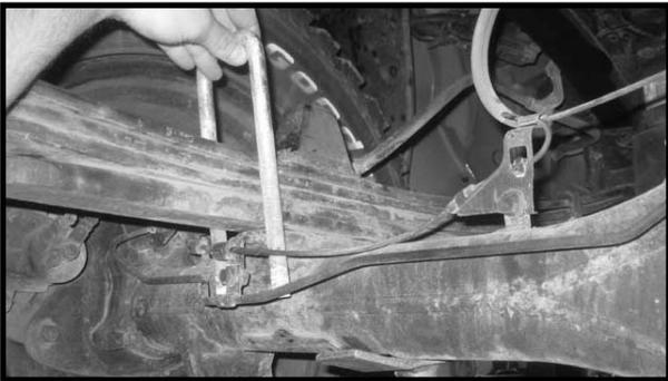
40. Carefully lower down on both hydraulic floor jacks at the same time allowing enough room for the rear blocks to be installed. **Special note: Take special care not to over extend any brake lines and/or hoses.**
