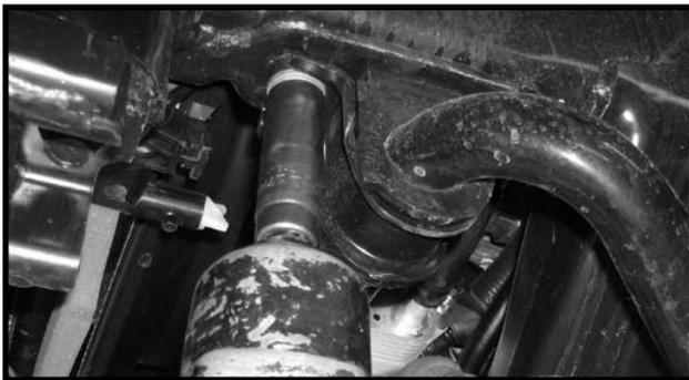
7. Place a pair of hydraulic floor jacks under the driver and passenger side lower control arm. Carefully raise up on them until they come into contact with the lower control arm.
