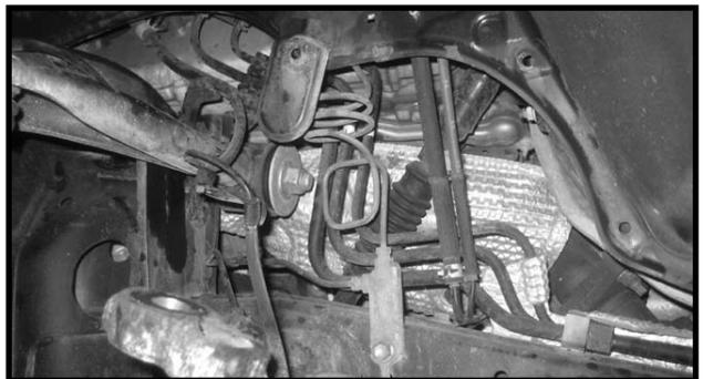
14. Working on the driver side, remove and save the hardware attaching the upper control arm to the OE location. The upper control arm may be discarded. Repeat procedure on the passenger side.
