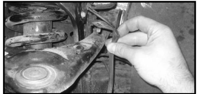
9. Working on the driver side, remove the (4) upper nuts holding the strut into the upper strut pocket. Save the hardware. Repeat procedure on the passenger side.
