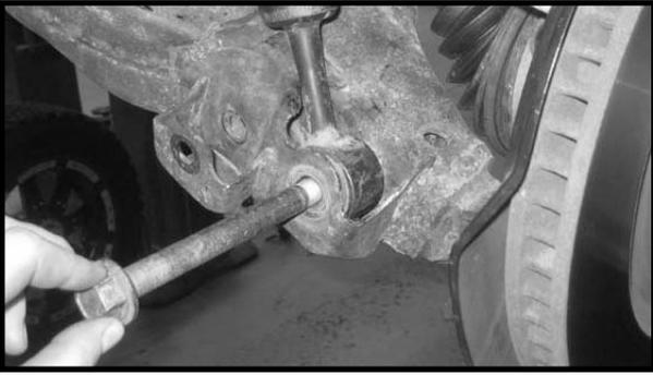
26. Working on the driver side, move back to the upper strut spacer and add some loctite on the bolts holding the modified strut into the upper location and torque to **35 ft lbs.** Repeat procedure on the passenger side.
