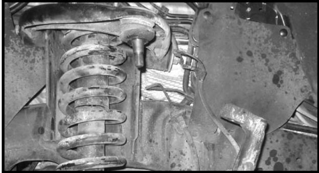
12. Working on the driver side, remove the lower mounting hardware that attaches the strut to the lower control arm. Save the hardware. Carefully lower down on the hydraulic floor jack allowing removal of the strut easier. Remove the strut and set aside. Repeat procedure on the passenger side.
