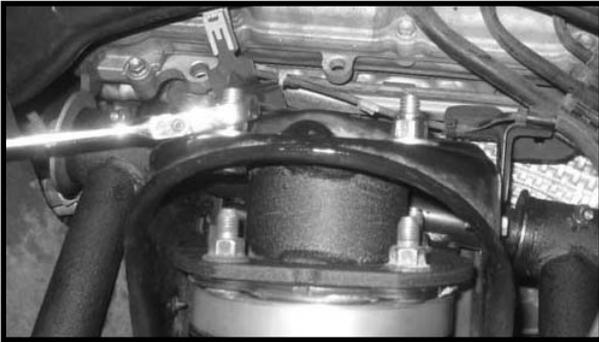
27. Remove the new cotter pin, castle nut and washer from each new upper control arm and set aside.
