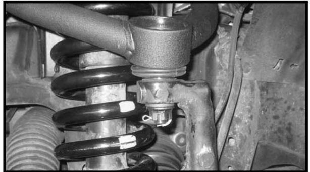
29. Locate (2) 1/4" unitorque nuts and (2) 1/4" USS flat washers from hardware bag 54070NB1. Working on the driver side, install the ABS line brake to the new upper control arm and secure using the new hardware. Make sure to use loctite and torque to **5 ft lbs.** Repeat procedure on the passenger side.
