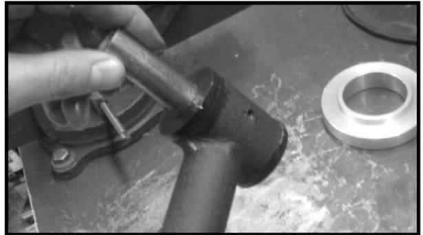
16. Locate the new sert fittings from hardware bag 54070NB1. Install the new sert fittings into the new upper control arms. **Special note: Make sure not to over tighten and also make sure that the sert fitting is facing towards the outside of the vehicle. This will make for easier access when using a grease gun.**
