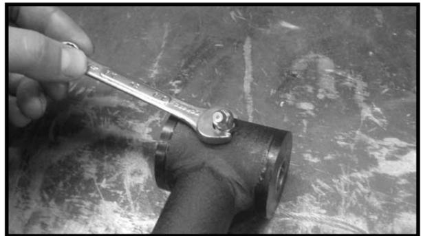
17. Locate (4) over size washers out of hardware bag 54070NB. Working on the driver side, install the new upper control arm into the OE pocket using the OE hardware along with the new over size washers. **Special note: The over size washers will be installed on the inside of the arm as it attaches to both the front and rear mounts. Make sure to use Loctite and torque upper control arm bolt to 100 ft lbs. Repeat procedure on the passenger side.**
