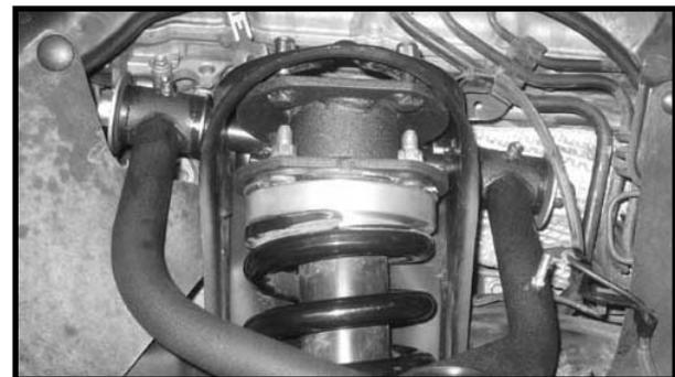
25. Working on the driver side, secure the bottom portion of the strut to the lower control arm using the OE hardware. Make sure to use loctite and torque to **150 ft lbs.** Repeat procedure on the passenger side.
