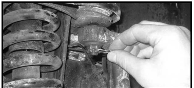
11. Working on the driver side, loosen but do not remove the castle nut holding the upper control arm to the knuckle. With a hammer, hit the knuckle to break the taper. Once the taper has been broken, remove the castle nut and discard. Separate the upper control arm from the knuckle. Repeat procedure on the passenger side.
