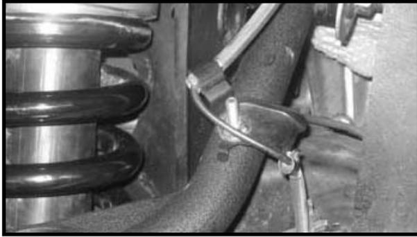
30. Locate the new sway bar relocation brackets. Also, locate (4) 12 mm x 60 mm bolts, (4) 12 mm flat washers and (4) 12 mm lock washers from hardware bag 54070NB1. Working on the driver side, install the new sway bar relocation bracket between the sway bar and the OE mount and secure using the new 12 mm hardware. **Do not tighten at this point.** Repeat procedure on the passenger side. Once both sides have been attached add loctite on each new 12 mm bolt and torque to **65 ft lbs.**
