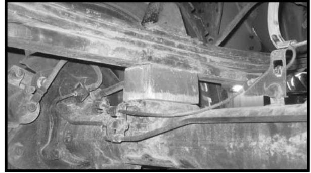
42. Locate (4) 9/16" x 2 9/16" x 9 5/8" square u-bolts. Locate (8) 9/16" u-bolt high nuts and (8) u-bolt washers from hardware bag 916NW. Also, locate the lower u-bolt plates. Working on the driver side, install the new u-bolts into the stock location and secure using the new 9/16" high nuts and washers. **Special note: If need be, cut off the excess threads off each leg of the newly installed u-bolts.** Torque to **120 ft lbs.** Repeat procedure on passenger side.
