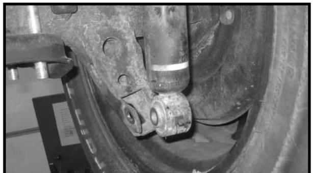
38. Working on the driver side, remove the OE emergency brake cable bracket from the axle. Save the hardware. Repeat procedure on the passenger side.
