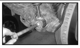
26. Working on the driver side, move back to the upper strut spacer and add some loctite on the bolts holding the modified strut into the upper location and torque to **35 ft lbs.** Repeat procedure on the passenger side.
