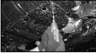
3. Working on the driver side, remove the hardware that attaches the front portion of the differential to the OE mounts. Save the over size washer on the head side of the bolt. Repeat procedure on the passenger side.
