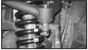
29. Locate (2) 1/4" unitorque nuts and (2) 1/4" USS flat washers from hardware bag 54070NB1. Working on the driver side, install the ABS line brake to the new upper control arm and secure using the new hardware. Make sure to use loctite and torque to **5 ft lbs.** Repeat procedure on the passenger side.
