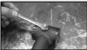
17. Locate (4) over size washers out of hardware bag 54070NB. Working on the driver side, install the new upper control arm into the OE pocket using the OE hardware along with the new over size washers. Special note: The over size washers will be installed on the inside of the arm as it attaches to both the front and rear mounts. Make sure to use Loctite and torque upper control arm bolt to 100 ft lbs. Repeat procedure on the passenger side.
