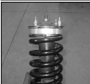
22. Locate the new upper strut spacer. Install the new upper strut spacer to the modified coil over and secure using the OE hardware. Make sure to use loctite and torque to 45 ft. lbs. Special note: There is a flat spot on the new spacer and this will be installed on the coil over facing towards the outside of the vehicle. Place the driver side strut aside for later installation into the vehicle.
