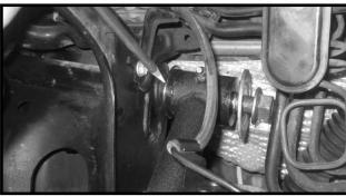
mounted strut compressor be used when performing tor from the bearing plate and discard. Install the new prethe steps that talk about installing the pre-load spacer load spacer to the bearing plate install it to the OE coil over into the strut. If you do not have a wall mounted strut using the OE hardware. Make sure to use loctite and torque compressor, please have these steps performed by your to 55 ft lbs. Special note: Make sure that the bearing local Toyota Dealership
