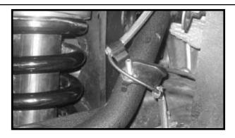
30. Locate the new sway bar relocation brackets. Also, locate (4) 12 mm x 60 mm bolts, (4) 12 mm flat washers and (4) 12 mm lock washers from hardware bag 54070NB1. Working on the driver side, install the new sway bar relocation bracket bracket between the sway bar and the OE mount and secure using the new 12 mm hardware. Do not tighten at this point. Repeat procedure on the passenger side. Once both sides have been attached add loctite on each new 12 mm bolt and torque to 65 ft lbs.
