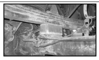
42. Locate (4) 9/16" x 2 9/16" x 9 5/8" square u-bolts. Locate (8) 9/16" u-bolt high nuts and (8) u-bolt washers from hardware bag 916NW. Also, locate the lower u-bolt plates. Working on the driver side, install the new u-bolts into the stock location and secure using the new 9/16" high nuts and washers. Special note: If need be, cut off the excess threads off each leg of the newly installed u-bolts. Torque to 120 ft lbs. Repeat procedure on passenger side.
