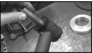
16. Locate the new sert fittings from hardware bag 54070NB1. Install the new sert fittings into the new upper control arms. Special note: Make sure not to over tighten and also make sure that the sert fitting is facing towards the outside of the vehicle. This will make for easier access when using a grease gun.
