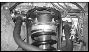
25. Working on the driver side, secure the bottom portion of the strut to the lower control arm using the OE hardware. Make sure to use loctite and torque to **150 ft lbs**. Repeat procedure on the passenger side.
