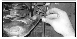
9. Working on the driver side, remove the (4) upper nuts holding the strut into the upper strut pocket. Save the hardware. Repeat procedure on the passenger side.
