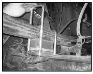
43. Locate the new emergency brake cable extension brackets. Working on the driver side, install the new emergency brake cable bracket to the rear axle using the OE hardware. Do not tighten at this point. Repeat procedure on the passenger side.
