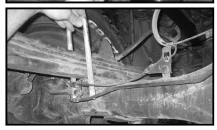
40. Carefully lower down on both hydraulic floor jacks at the same time allowing enough room for the rear blocks to be installed. Special note: Take special care not to over extend any brake lines and/or hoses.
