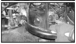
15. Locate the new upper control arms. Locate (8) poly bushings and (4) S10239 sleeves from hardware bag 54070NB. Install the new bushings and sleeves into the new upper control arms. Special note: Make sure to use a fair amount of lithium or moly base grease before installing the new bushings and sleeves into the control arms. This will increase the life of the bushing as well as help prevent squeaking.
