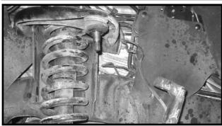
12. Working on the driver side, remove the lower mounting hardware that attaches the strut to the lower control arm. Save the hardware. Carefully lower down on the hydraulic floor jack allowing removal of the strut easier. Remove the strut and set aside. Repeat procedure on the passenger side.
