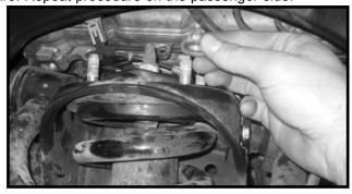
10. Working on the driver side, remove the cotter pin from the castle nut holding the upper control arm to the knuckle. The cotter pin may be discarded. Repeat procedure on the passenger side.
