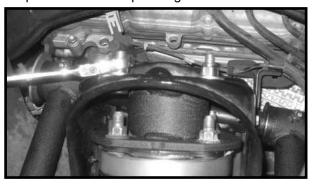
27. Remove the new cotter pin, castle nut and washer from each new upper control arm and set aside.
