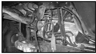
14. Working on the driver side, remove and save the hardware attaching the upper control arm to the OE location. The
